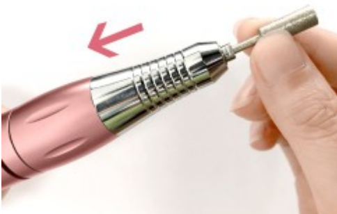
Step 3: Change to the required polishing drill bit
