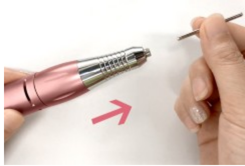
Step 2: Pull out original blank drill bit and remove it
