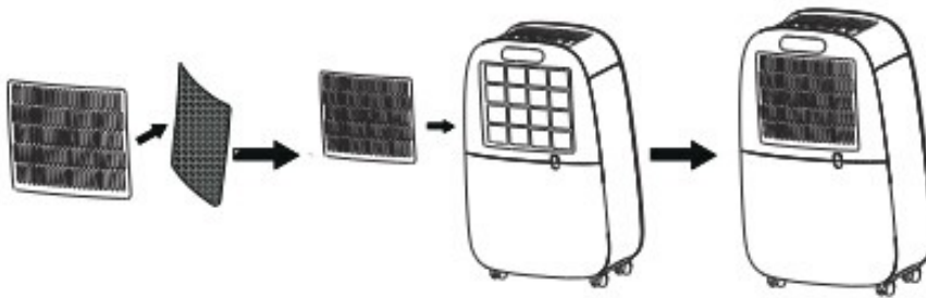
Pic6. Re-assembly the air filter.
